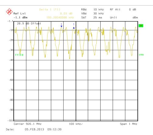
Channel Separation equal to the 20 dB bandwidth: 100.200 kHz
