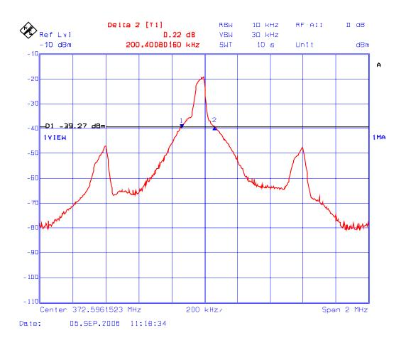
Plot #2: 20 dB Bandwidth, FSK Test Frequency: 372.6 MHz
