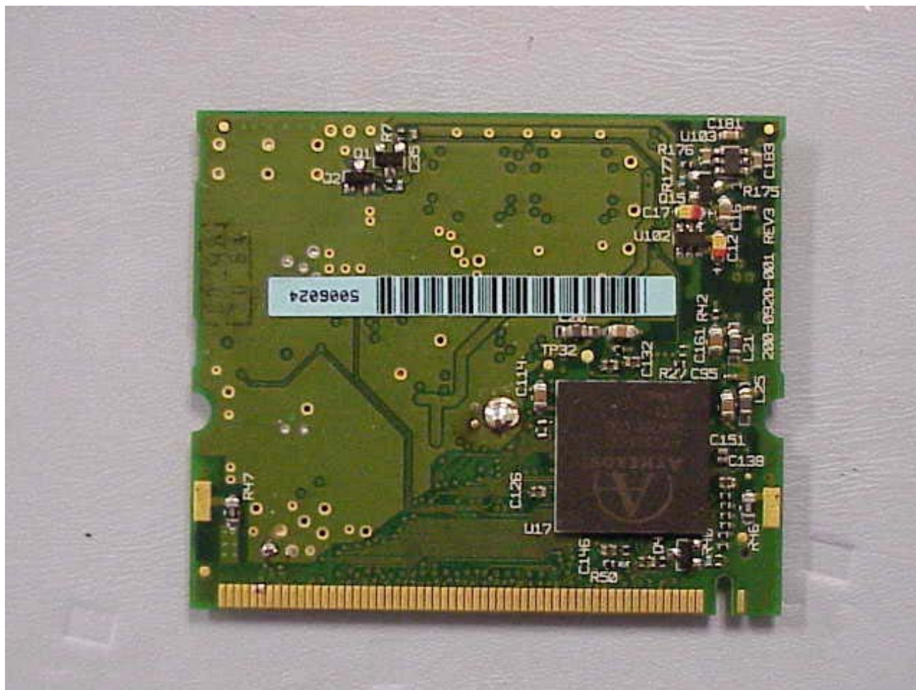
Back Side of MINI PCI Card bus W/ Atheros Chip Set
