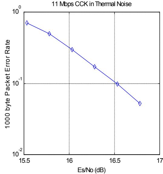
The reference PER is specified as 8%. The corresponding Es/No (signal to noise ratio per symbol) is 16.4 dB. The Es/No required to achieve the desired BER with maximum system implementation losses is 18.4 dB. The minimum processing gain is again, 10 dB, therefore:
