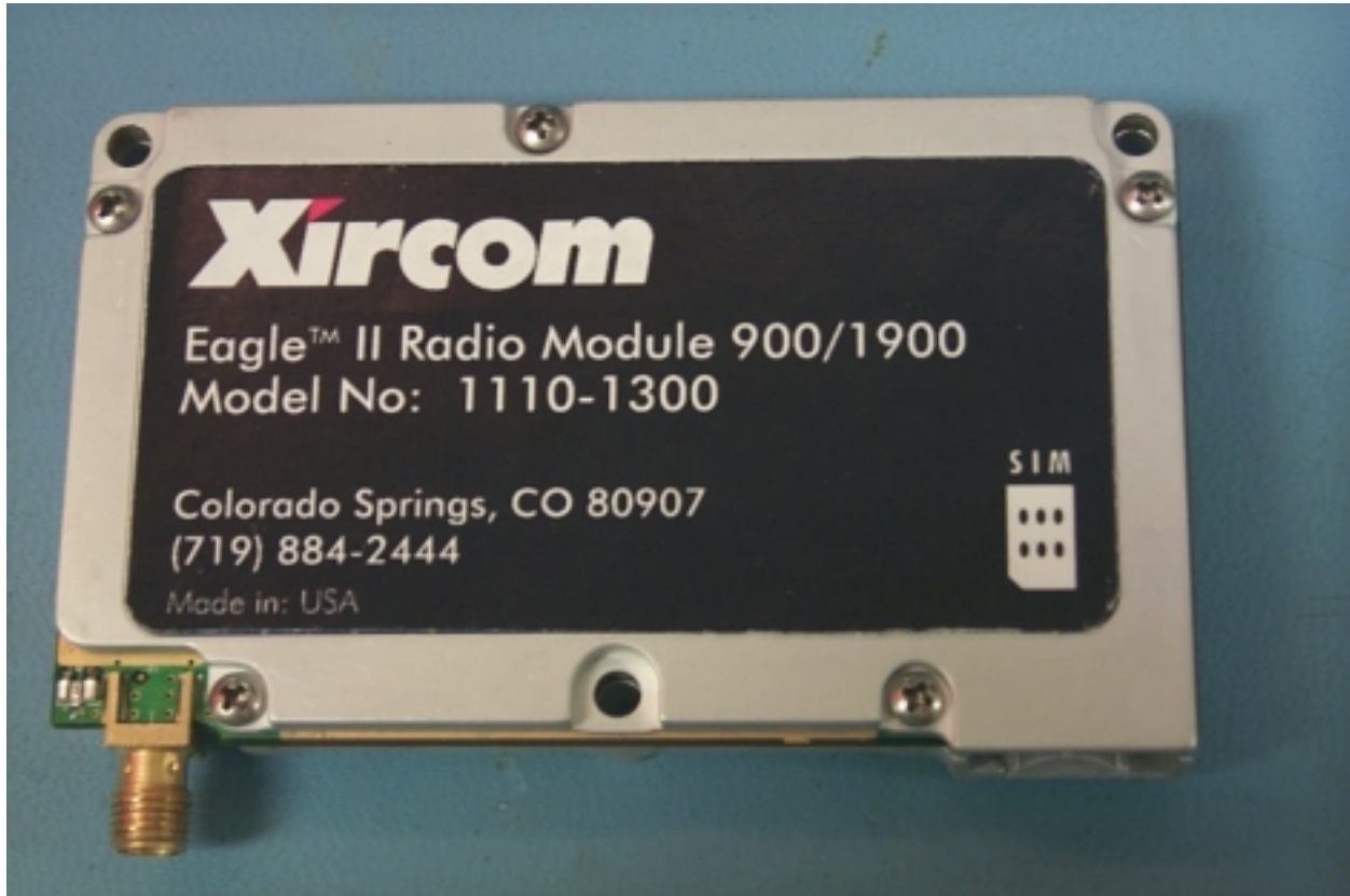
Photo 3. Top of Eagle II (shields in place).
