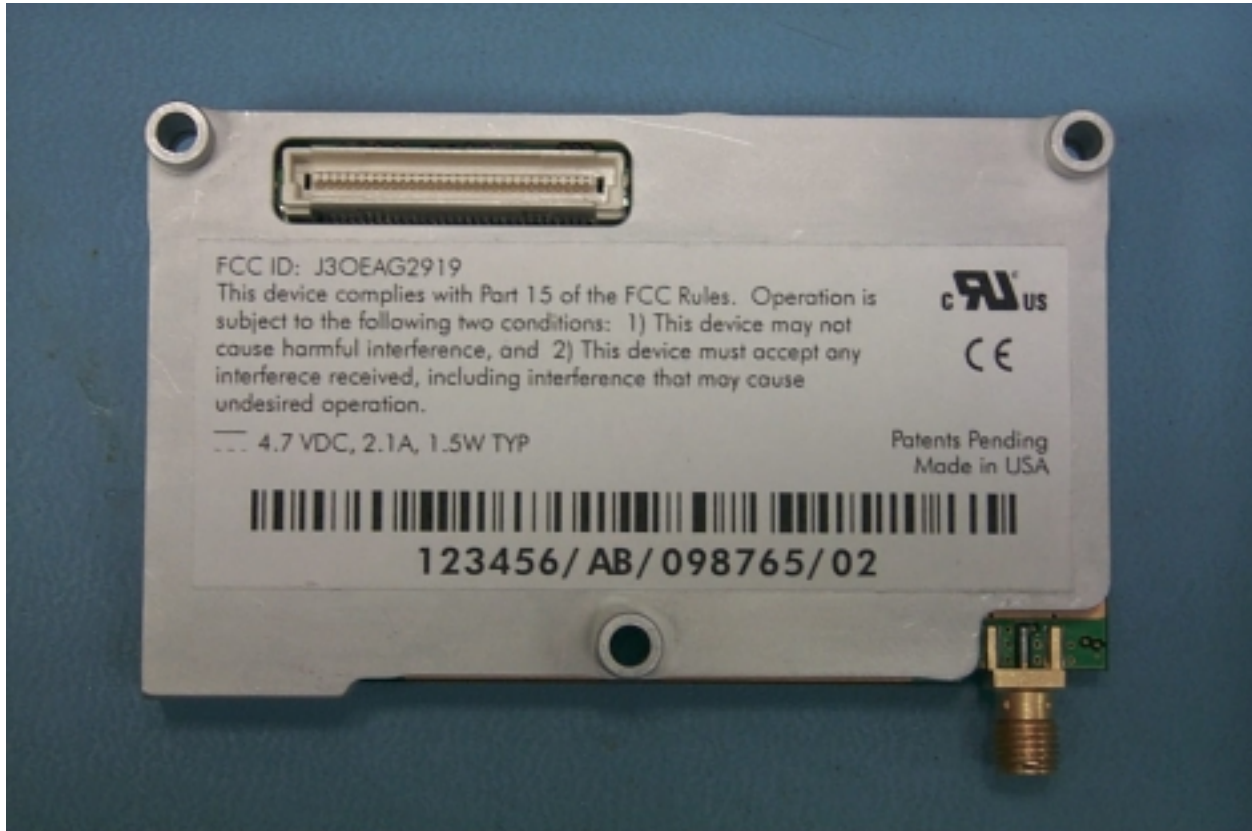
Photo 4. Bottom of Eagle II (shield in place).
