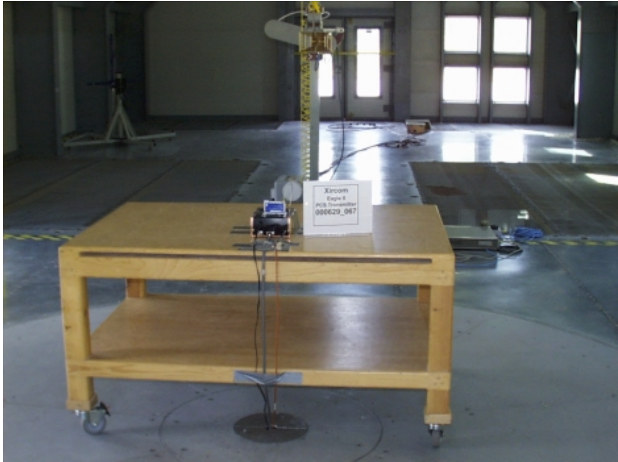
Figure E14.1. Radiated Emissions set-up at Criterion Technologies.
