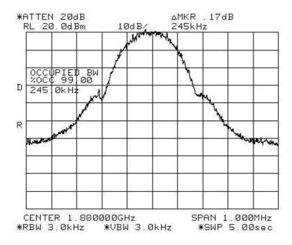
Figure E12.1. Sample measurement of occupied bandwidth.
