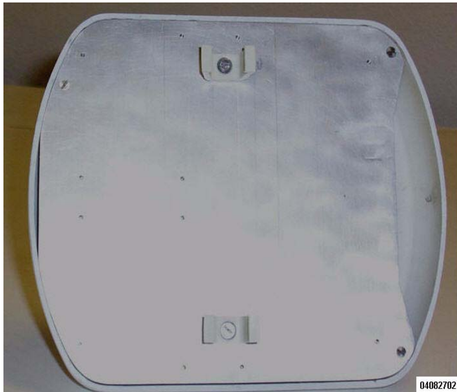
Figure - Airespace AP with Ceiling-Mount Clips Installed
