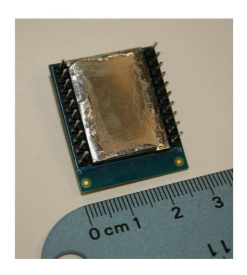
Figure 2: Bottom View of WPAN Module
