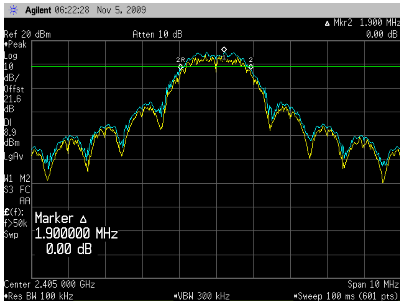
(Low Channel) Observed 6 dB Bandwidth is 1.9 MHz
