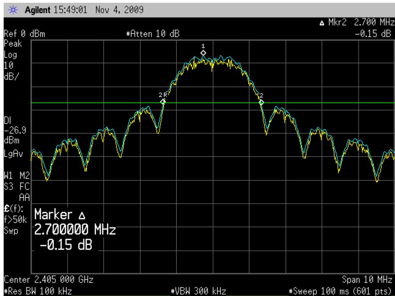
(Low Channel) Observed 20 dB Bandwidth is 2.7 MHz
