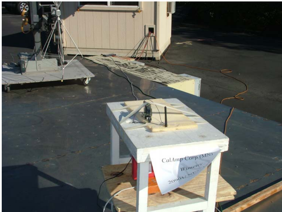
"Red Box" is test control box used to activate the radio and to change channel. It is turned off during radiated emission tests.
