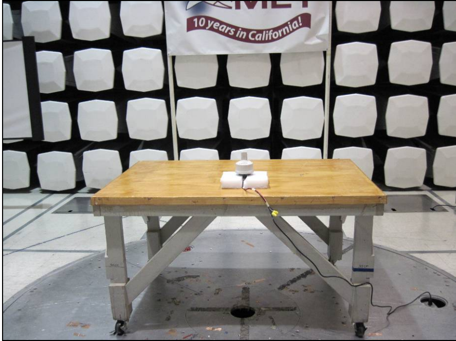
Photograph 3. Radiated Emissions, Test Setup
