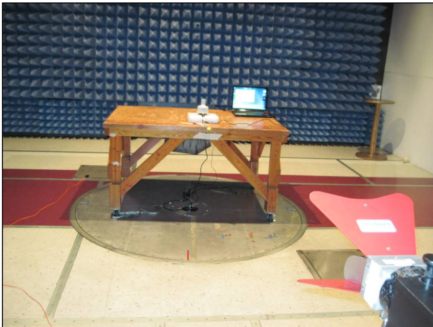
Photograph 10. Radiated Spurious Emissions, Test Setup, 1 GHz – 18 GHz
