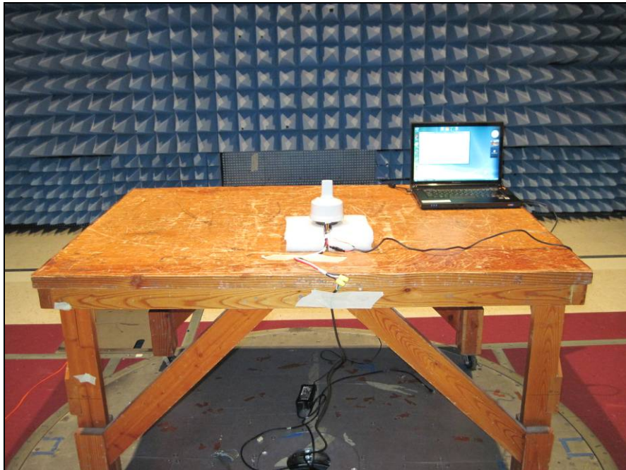
Photograph 8. Radiated Spurious Emissions, Test Setup
