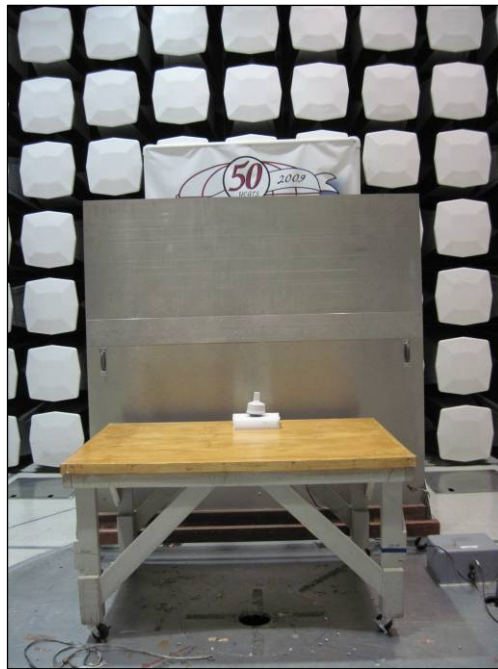
Photograph 6. Conducted Emissions, 15.207, Test Setup
