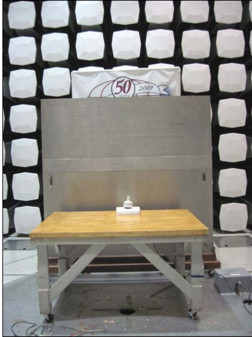
Photograph 1. Conducted Emissions, Test Setup
