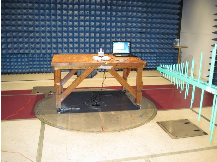
Photograph 9. Radiated Spurious Emissions, Test Setup, 30 MHz – 1 GHz
