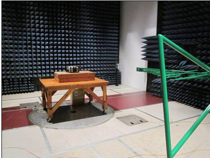
Photograph 3. Radiated Emissions, Test Setup, 30 MHz – 1 GHz
