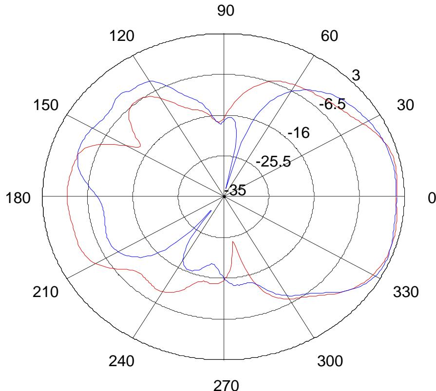
Plot 3. EVDO @ 1.9 GHz – elevation, co-polarization, 1-deg resolution
