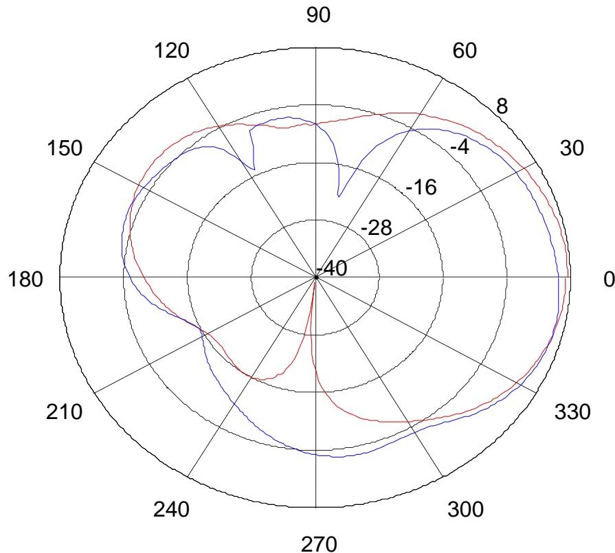
Plot 1. EVDO @ 850 MHz – elevation, co-polarization, 1-deg resolution
