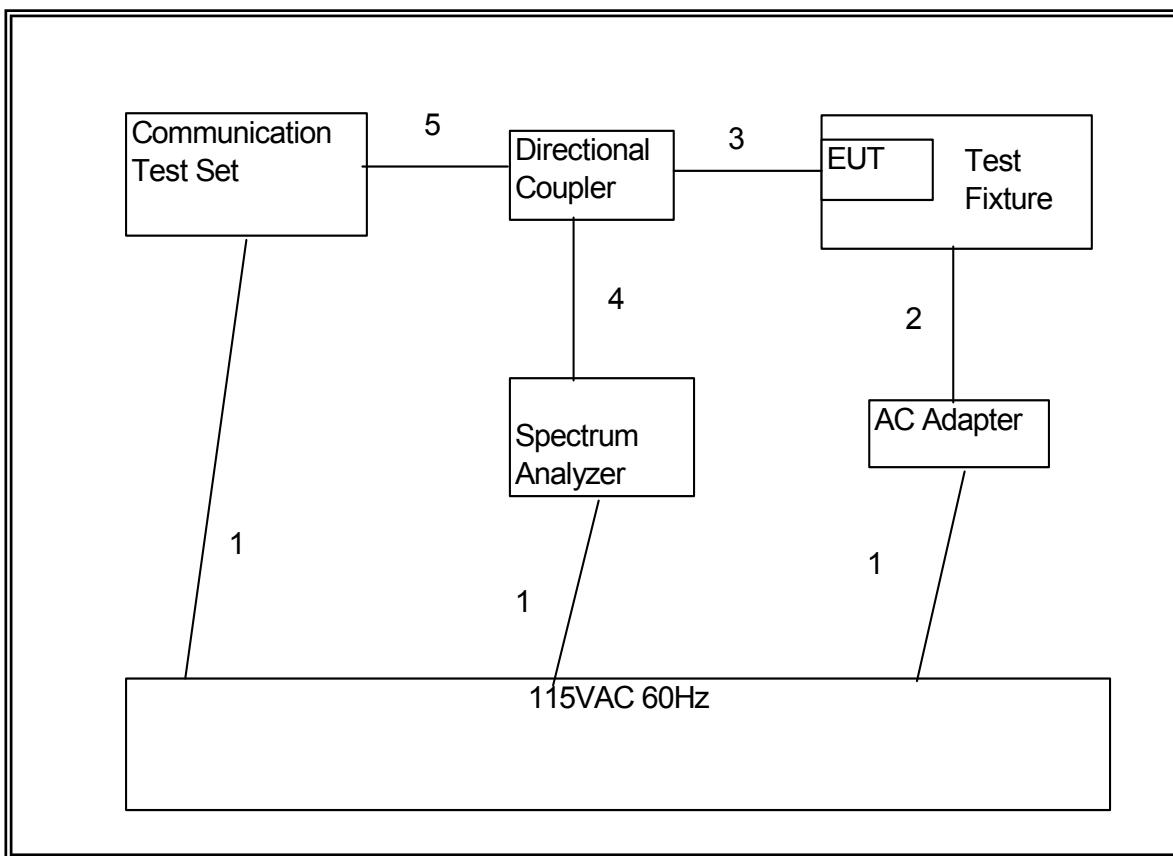
**SETUP DIAGRAM FOR RADIATED TESTS**
