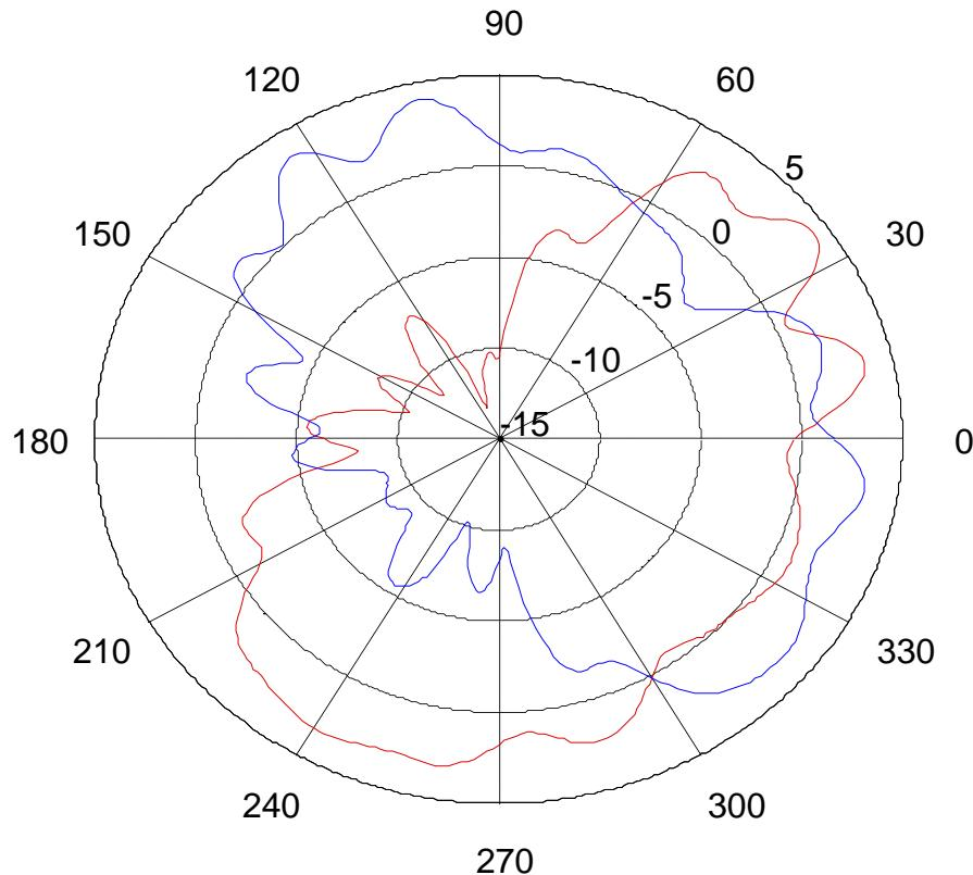
Plot 4. EVDO @ 1.9 GHz – azimuth, co-polarization, 1-deg resolution
