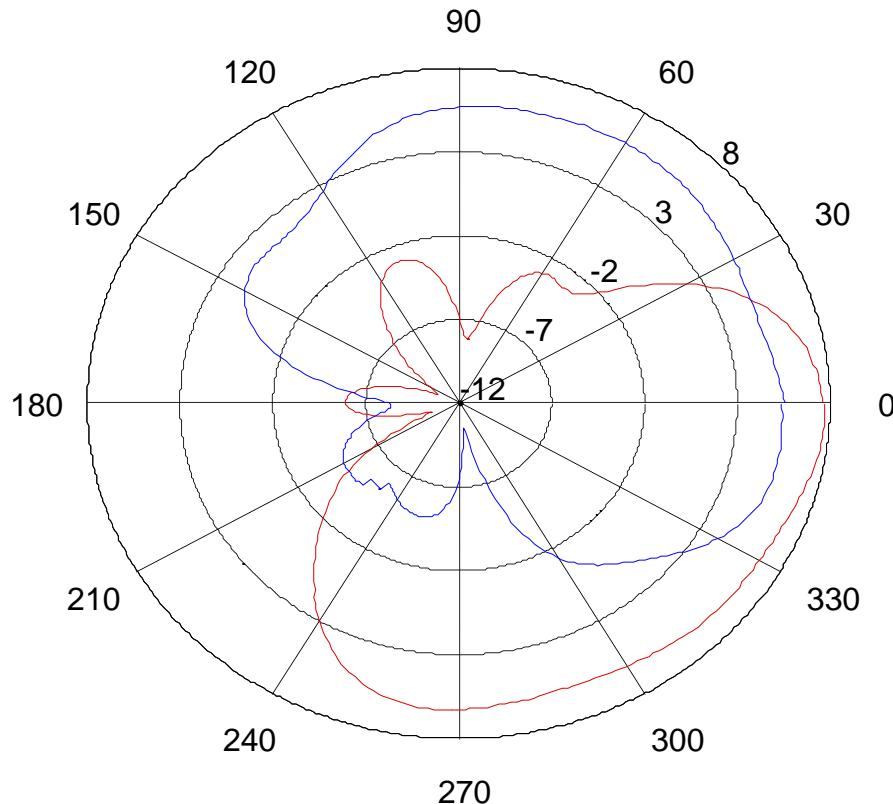
Plot 2. EVDO @ 850 MHz – azimuth, co-polarization, 1-deg resolution
