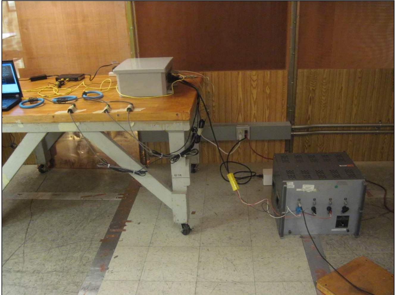
Photograph 1. Conducted Emissions, Test Setup
