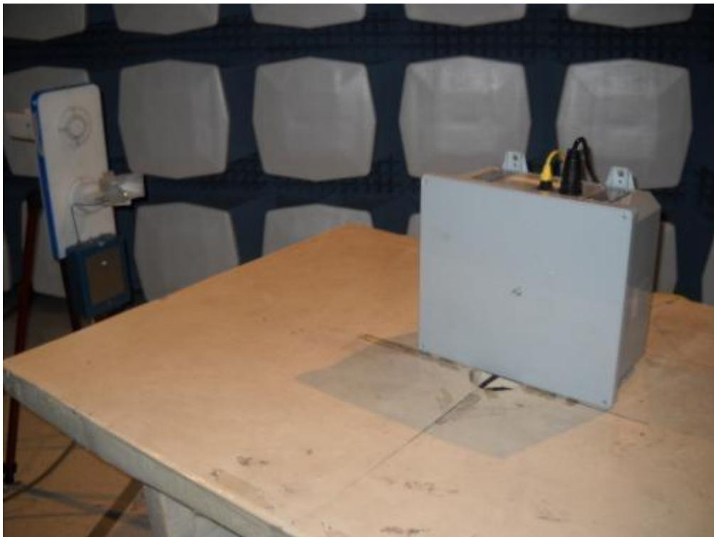
**Conducted Emissions Test Setup Pictures****Line Conducted emissions measurement-1**
