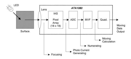
ATA1060XA is based on Optical Navigation Technology. It contains an Image Acquisition System (IAS), a Motion Vector Finding Processor (MVFP), a two-channel quadrature output.
