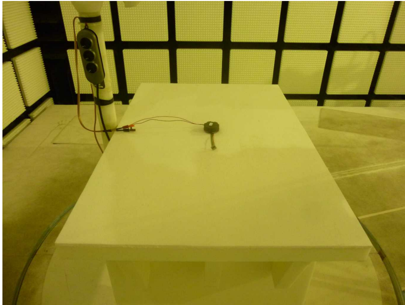
Photo 5: EUT at the anechoic chamber, loop antenna test setup
