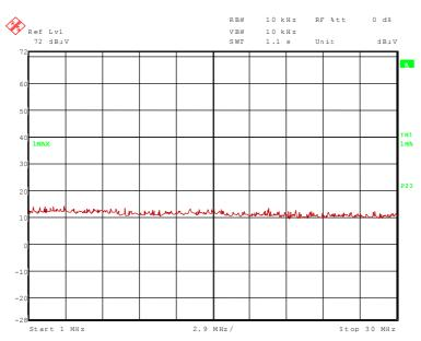
No significant frequencies above the noise floor of the system were found during the preliminary radiated emission test, so no measurements were carried out on the outdoor test site.
