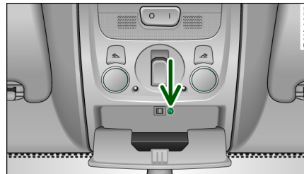
Fig. 22 Section from headliner: Unscrewing lighting unit
