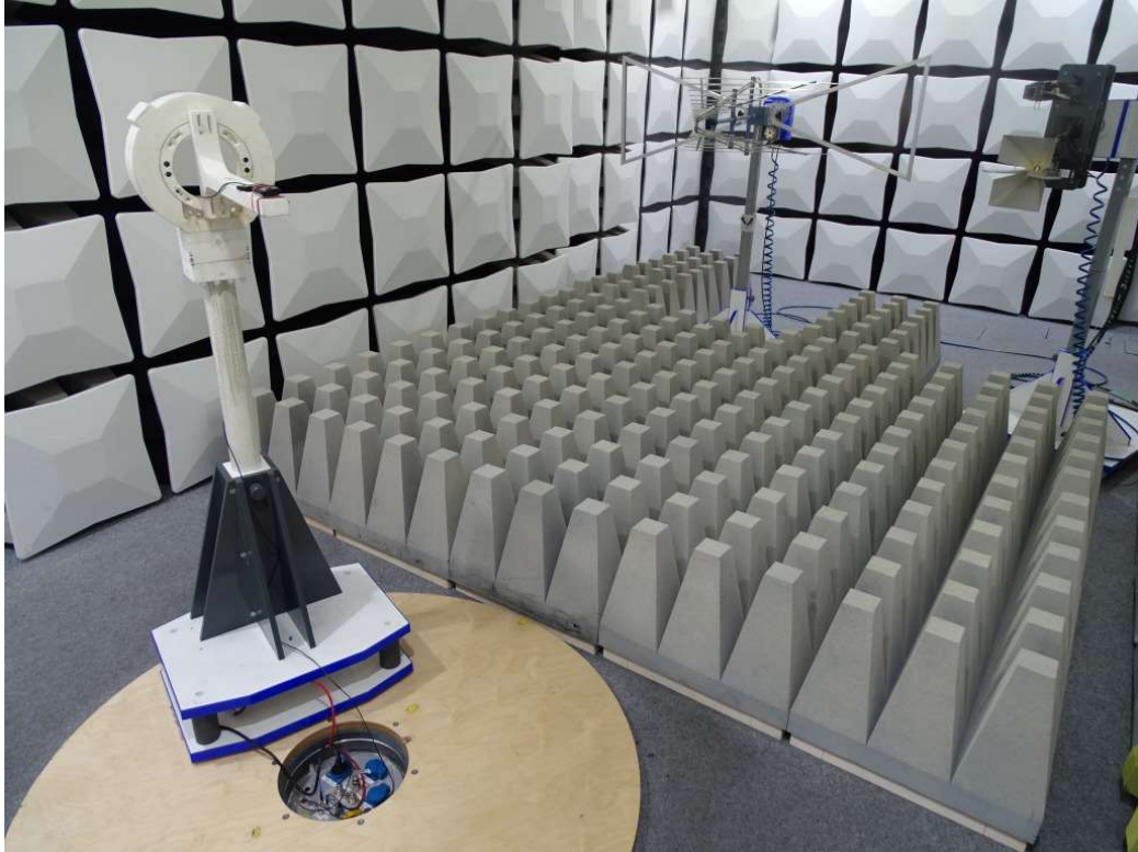
Photo 3: Test setup for radiated measurements above 1 GHz
