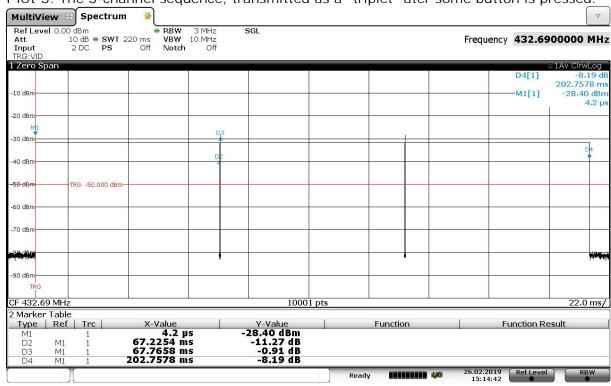
Plot 3. The 3-channel sequence, transmitted as a "triplet" ater some button is pressed.
