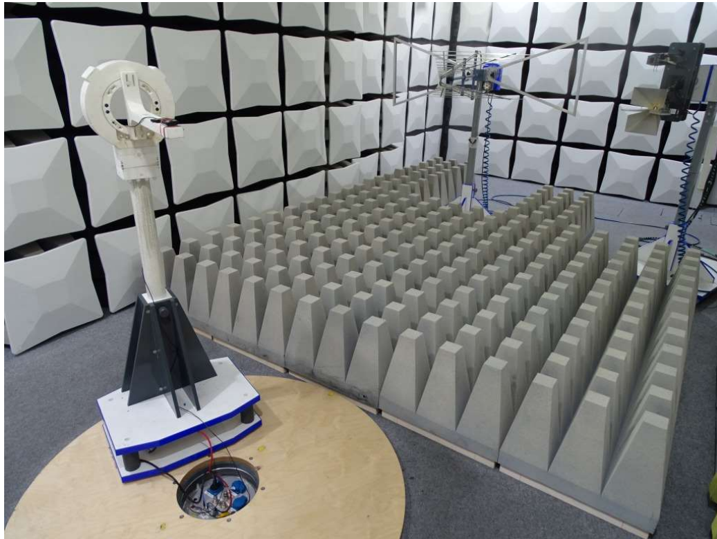
Photo 3: Test setup for radiated measurements above 1 GHz
