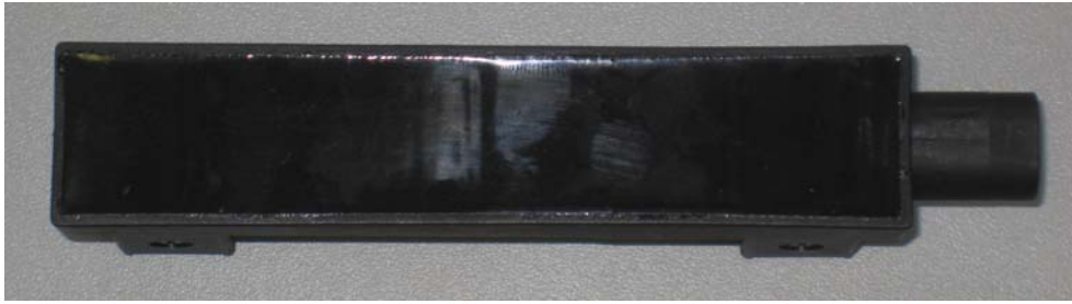
Rear view – LF antenna
