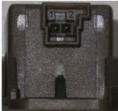
Connector view – LF antenna
