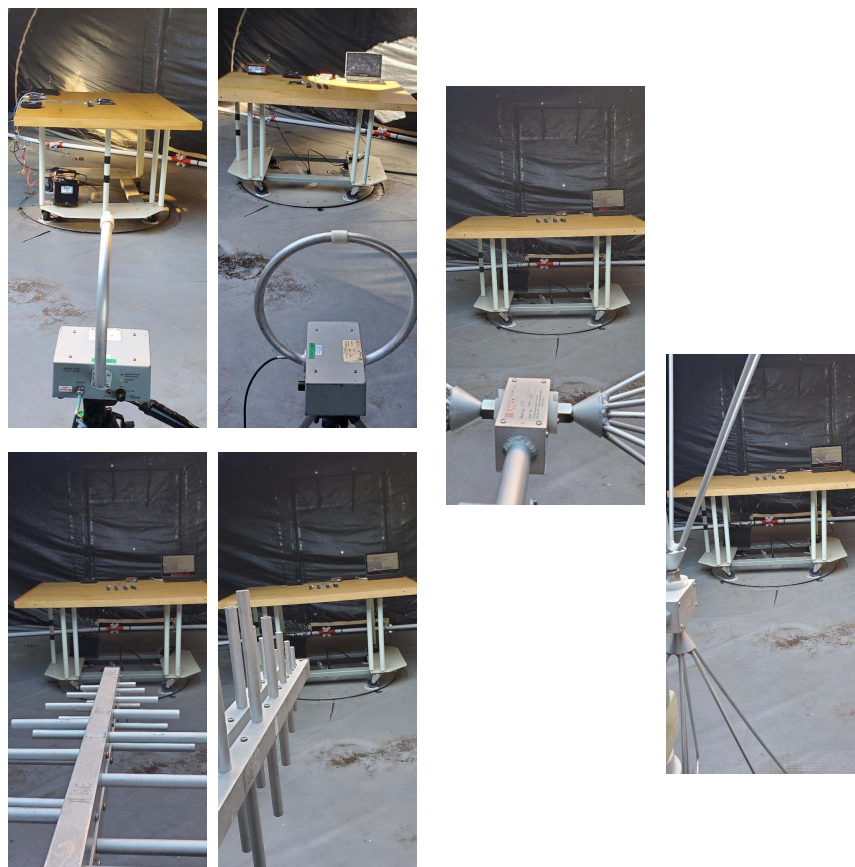
Figure 4: Radiated Emissions Test Setup Photograph(s).
