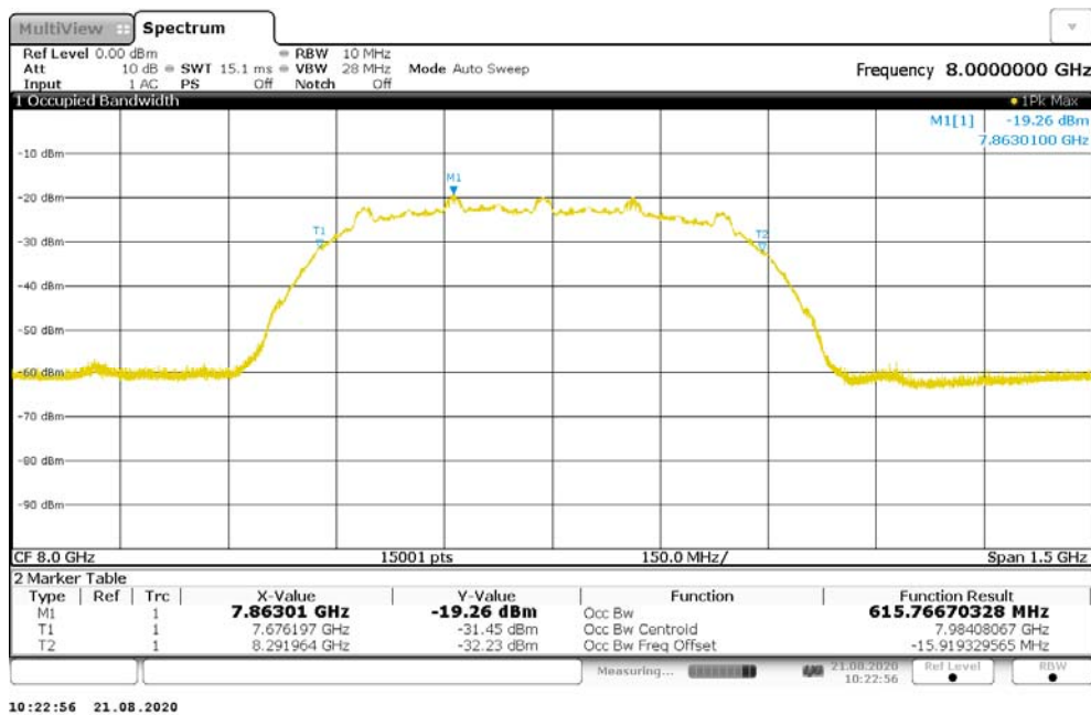
Figure 4 – 10 dB Bandwidth for Channel 9
