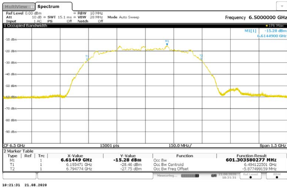
Figure 3 – 10 dB Bandwidth for Channel 5
