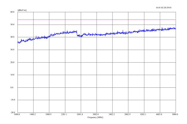
RBW/VBW 1 MHz, red line is limit at 3m distance.
