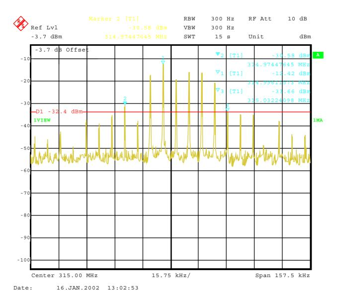
We used a small BW to determine the frequencies and a long sweep time to catch all signals. The red line is the -20 dB line (99.5 %) according to FCC standards.
