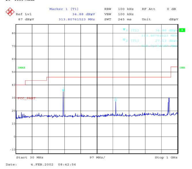
RBW/VBW 100 kHz. The measurements were made conducted at the antenna output.
