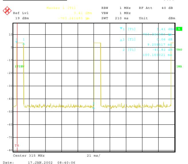
TX on-time is 9.25 ms, TX off + TX on is 100 ms. So we have a ratio of -10.34 dB between Peak and Average  $(10*\log(TX \text{ on}/(Tx \text{ on and off})))$
