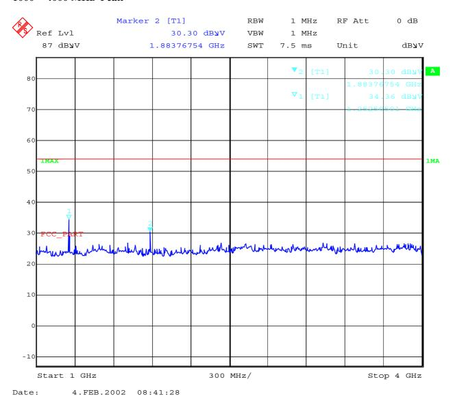
RBW/VBW 1000 kHz. The measurements were made conducted at the antenna output.
