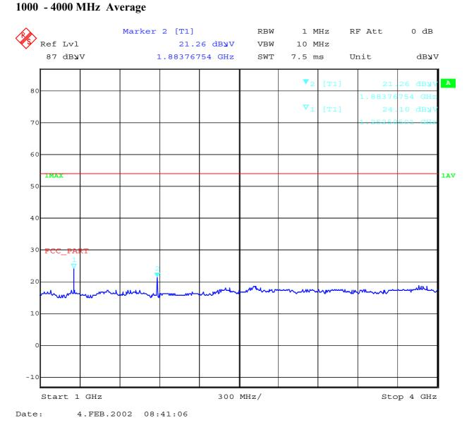
RBW/VBW 1000 kHz. The measurements were made conducted at the antenna output.
