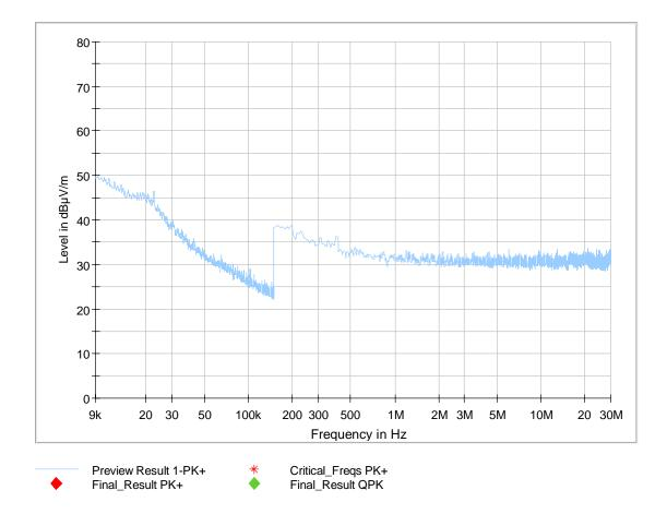
No significant frequencies above the noise floor of the system were found during the preliminary radiated emission test for PK3.
