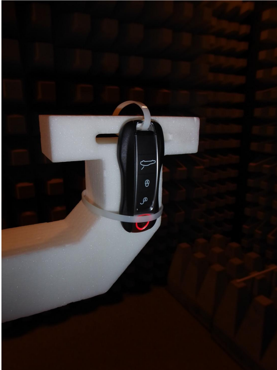
153783_4.JPG: Test setup fully anechoic chamber
