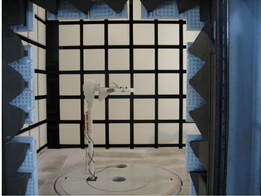
Photo 12: Test transceiver setup for 21 kHz keyless entry system
