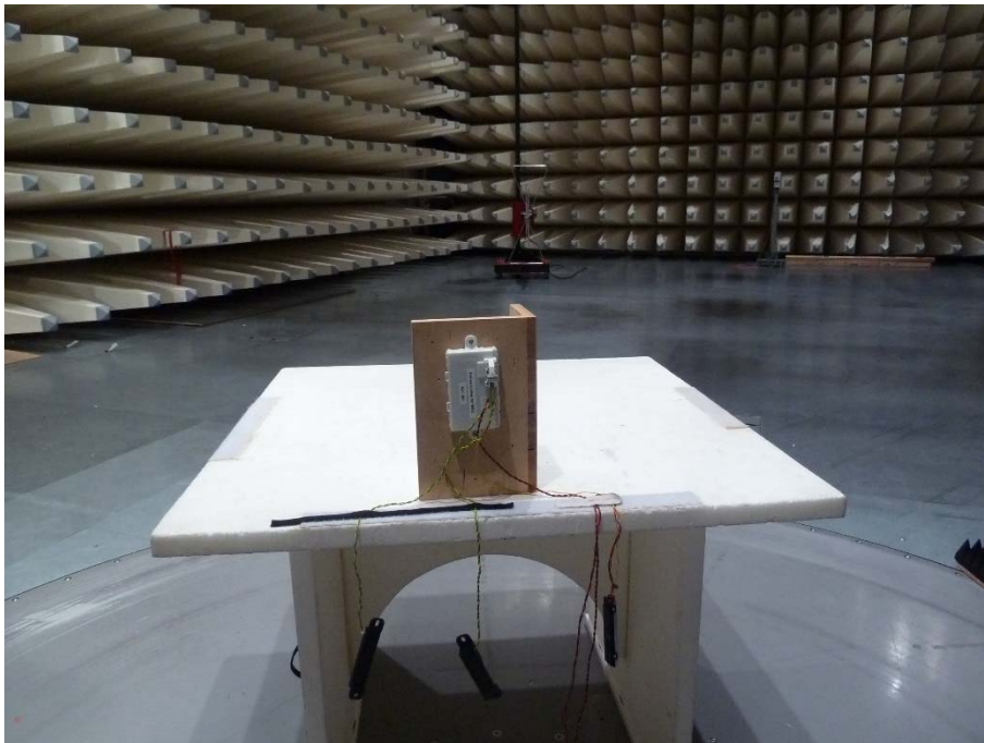
Photo 10: Test transceiver setup for 21 kHz keyless entry system
