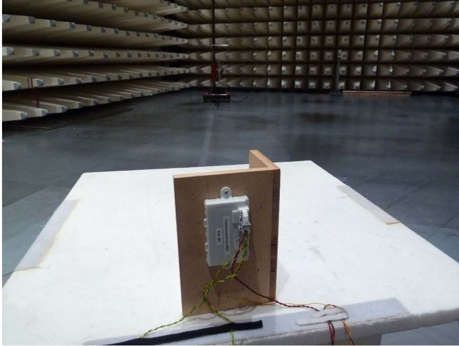
Photo 10: Test transceiver setup for 21 kHz keyless entry system
