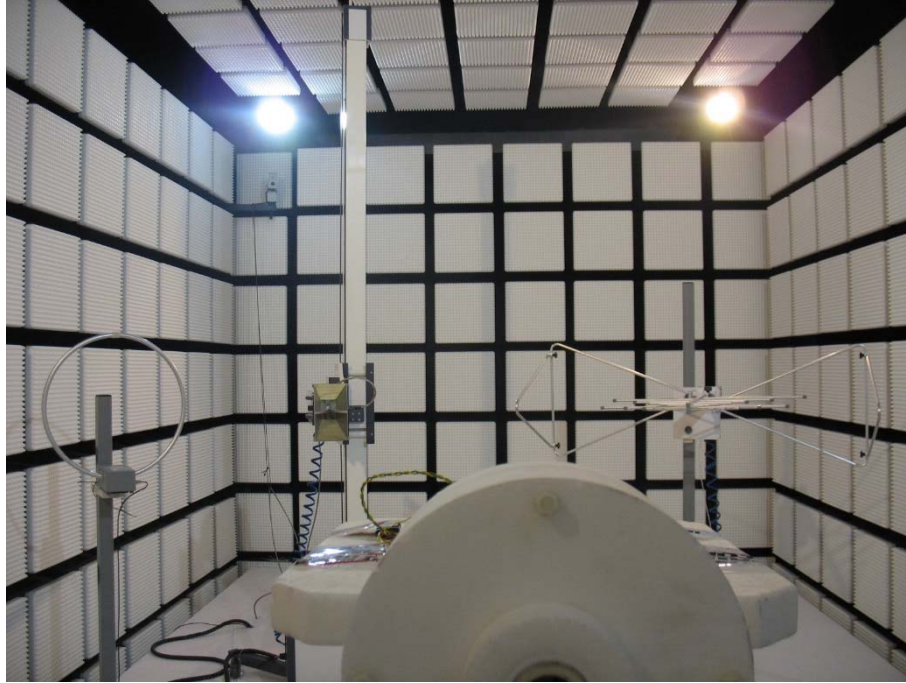
Photo 13: Test transceiver setup for 21 kHz keyless entry system
