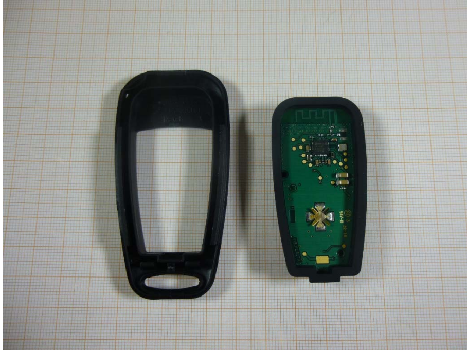
Photo 3: Front cover removed
