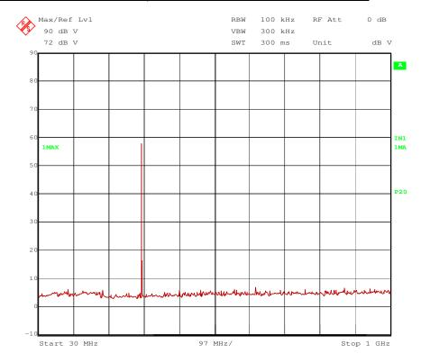
Only the nominal frequency of the transmitter was found during the preliminary radiated emission test:
