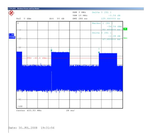
Based on the plot the duty cycle measured is 47.8 ms and is approximated to 48ms throughout this report.
