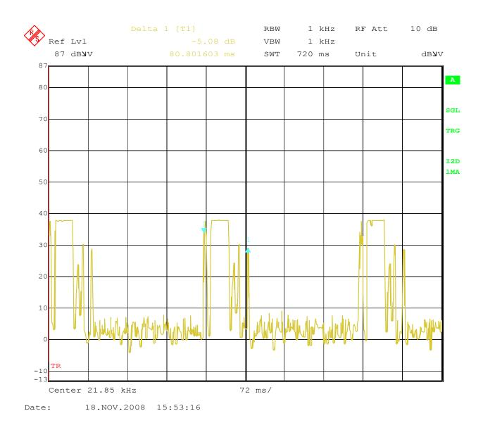
Duty cycle measured is 80.801603 ms, this is approximated to 81 ms and is used in calculations.
