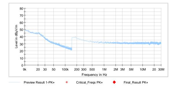
No significant frequencies above the noise floor of the system were found during the preliminary radiated emission test for AK2 Basis and AK2 Comfort.
