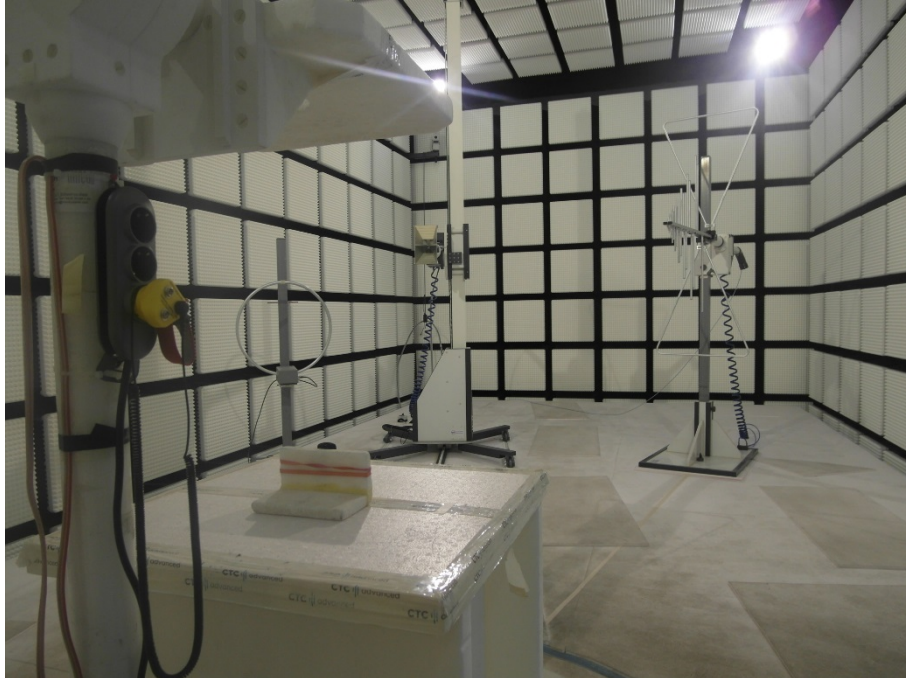
Photo 7: Setup for 9 kHz to 30 MHz
