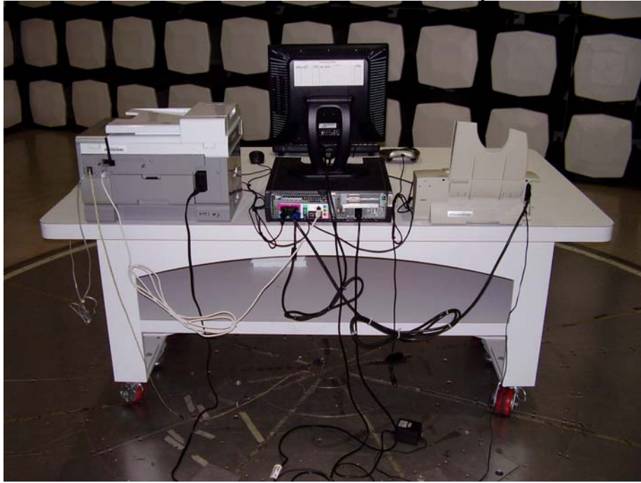
Figure 6. Test configuration for transmitter spurious emissions (rear view).
