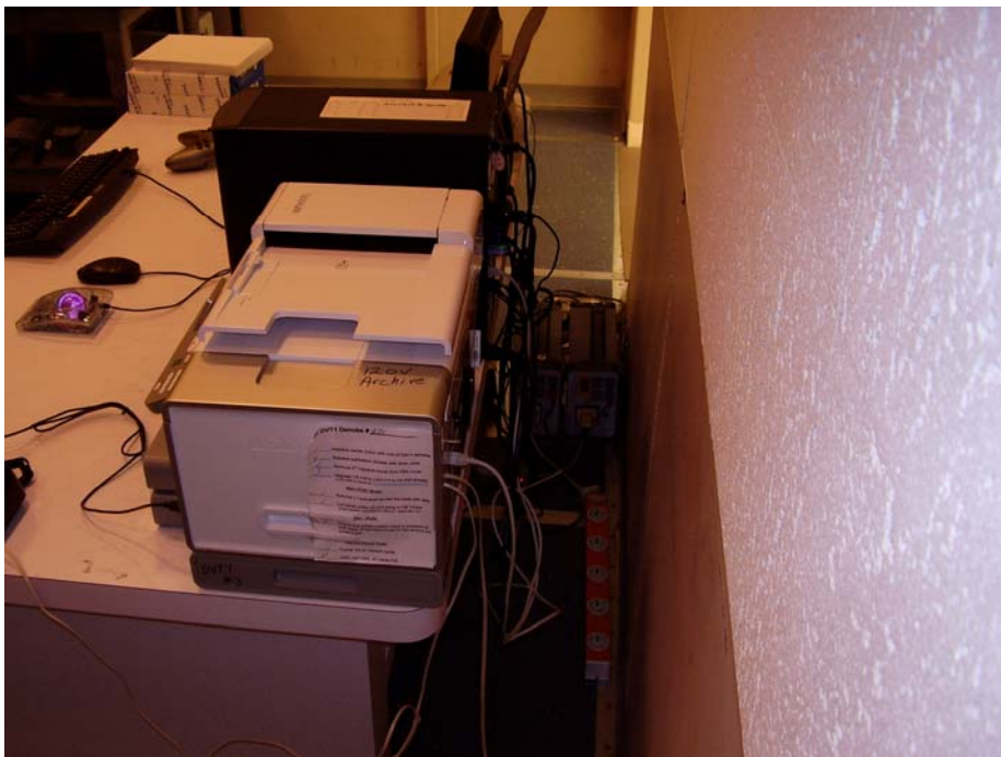
Figure 8. Test configuration for transmitter conducted emissions (side view).
