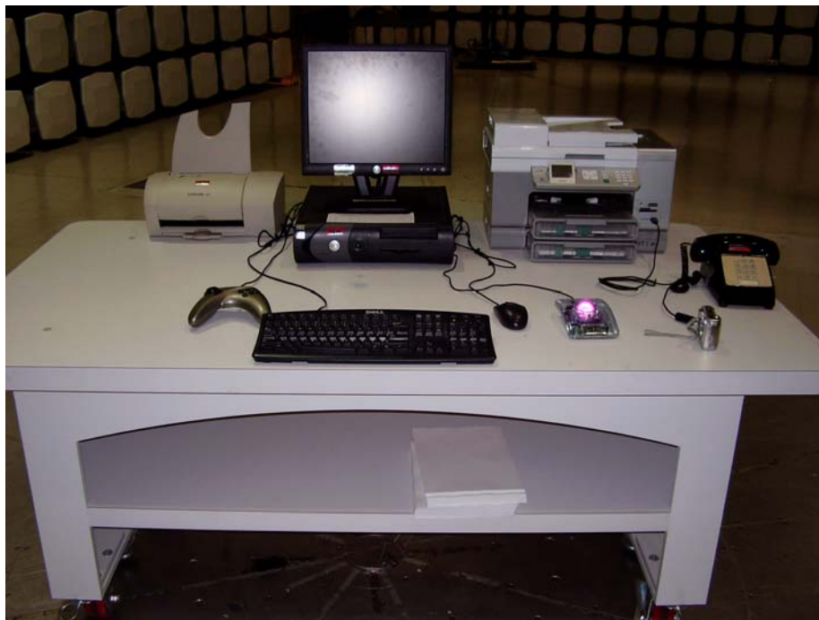
Figure 5. Test configuration for transmitter spurious emissions (front view).
