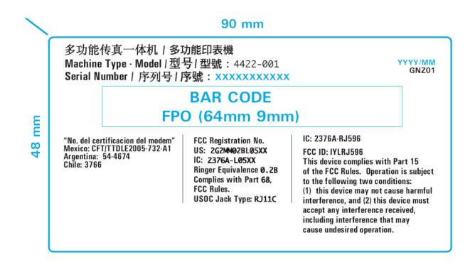
Wireless card is pre-installed at the factory. All wireless marks will be added to the machines ID label. This sample shows the label for the Lexmark X9350.
