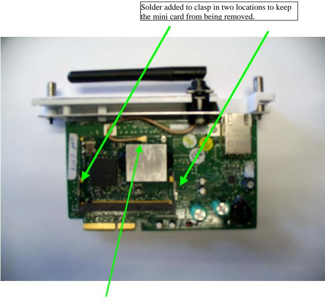
Solder added to antenna connection.
