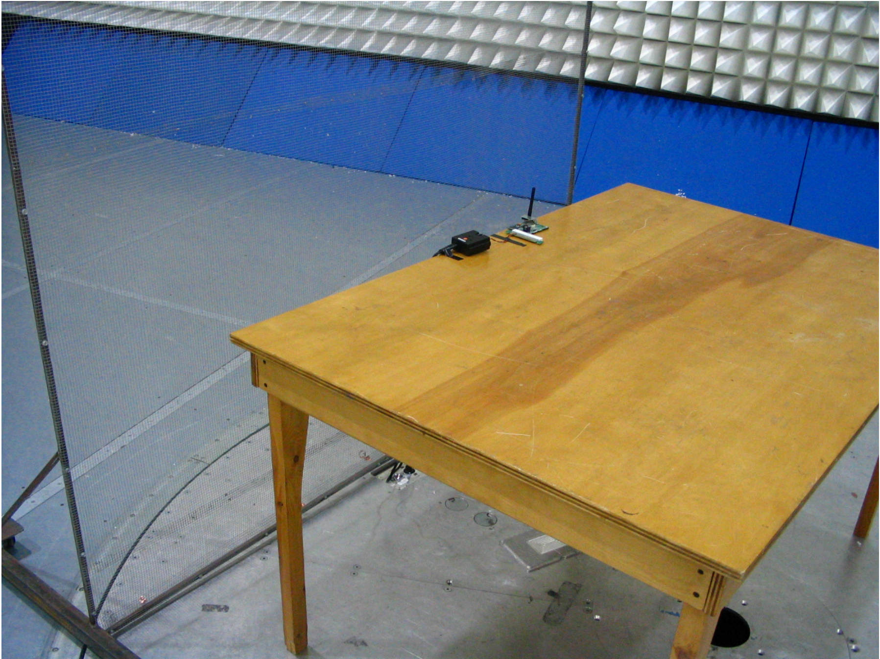
Figure 5: Conducted Emissions on the AC Power Input to the Power Supply (Front)
