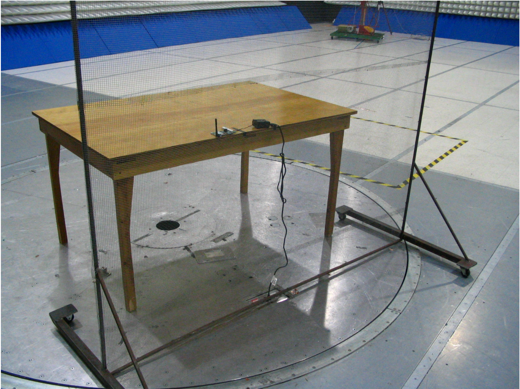
Figure 6: Conducted Emissions on the AC Power Input to the Power Supply (Back)
