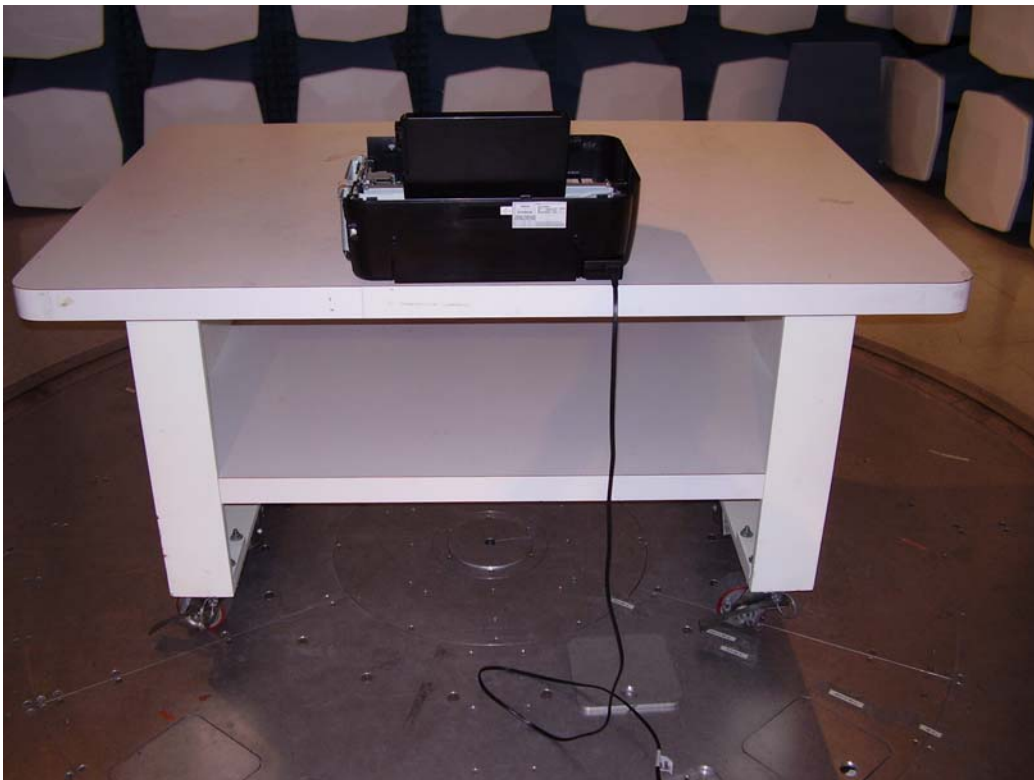
Figure 7. Test configuration for radiated emissions at f > 30 MHz (back view).
