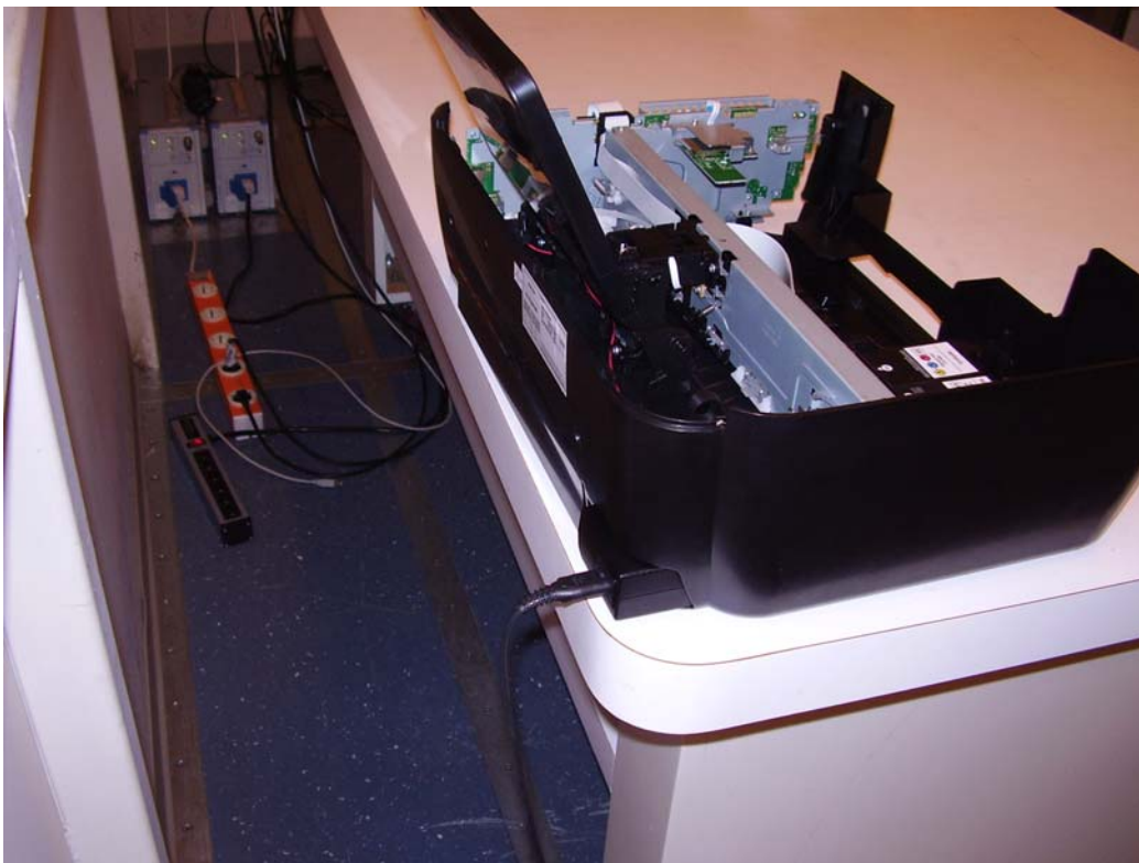
Figure 11. Test configuration for transmitter conducted emissions (side view).
