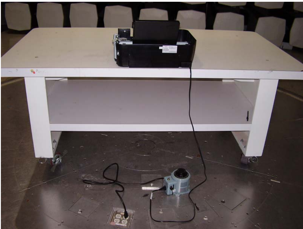
Figure 5. Test configuration for radiated emissions at f < 30 MHz (back view).
