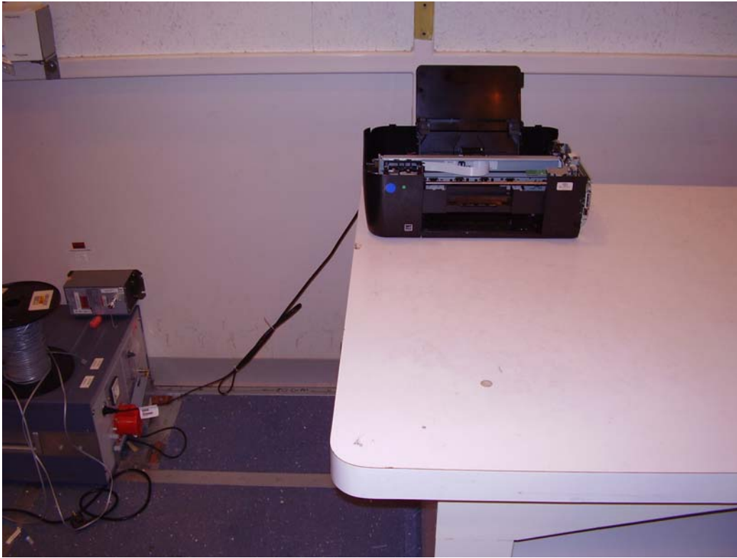
Figure 10. Test configuration for transmitter conducted emissions (front view).
