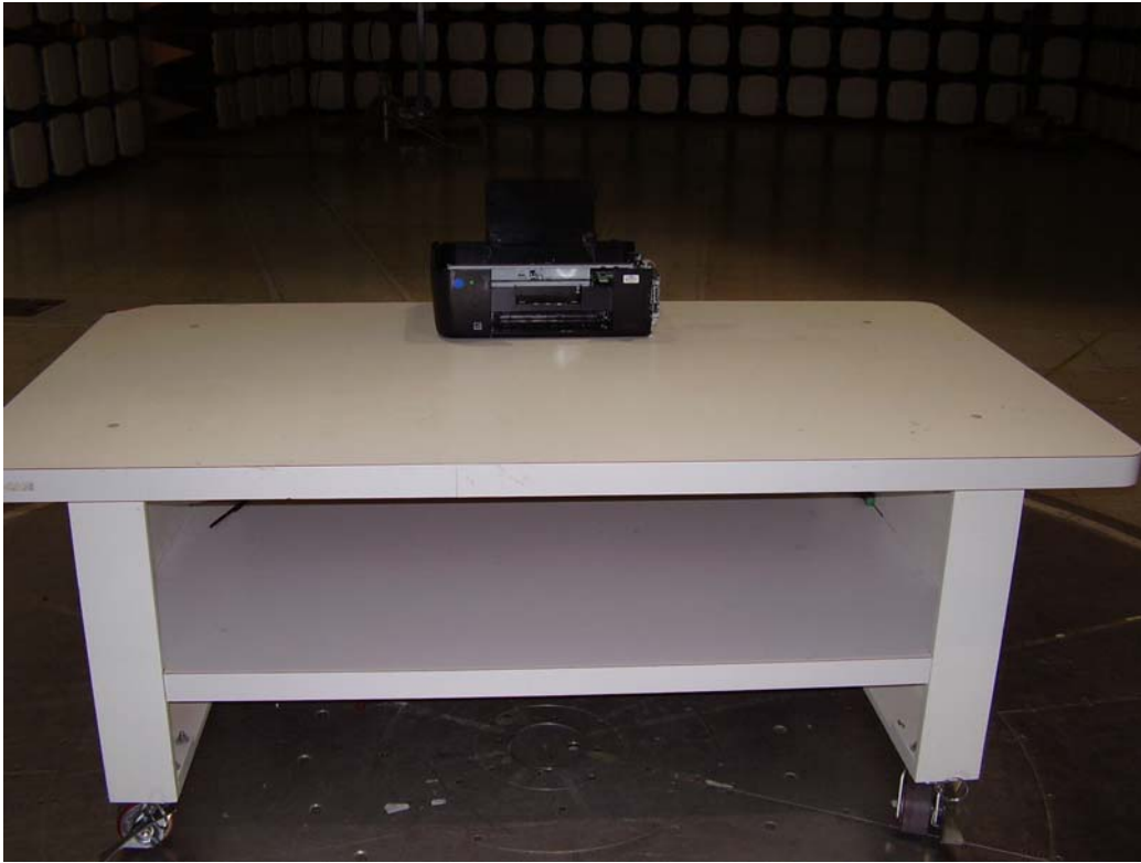
Figure 4. Test configuration for radiated emissions at f < 30 MHz (front view).
