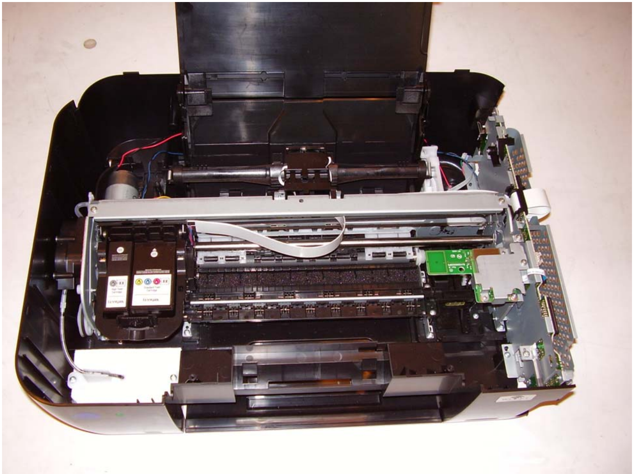
EUT mounted in printer engine frame with black plastic covers (tanks with tags to the left).
