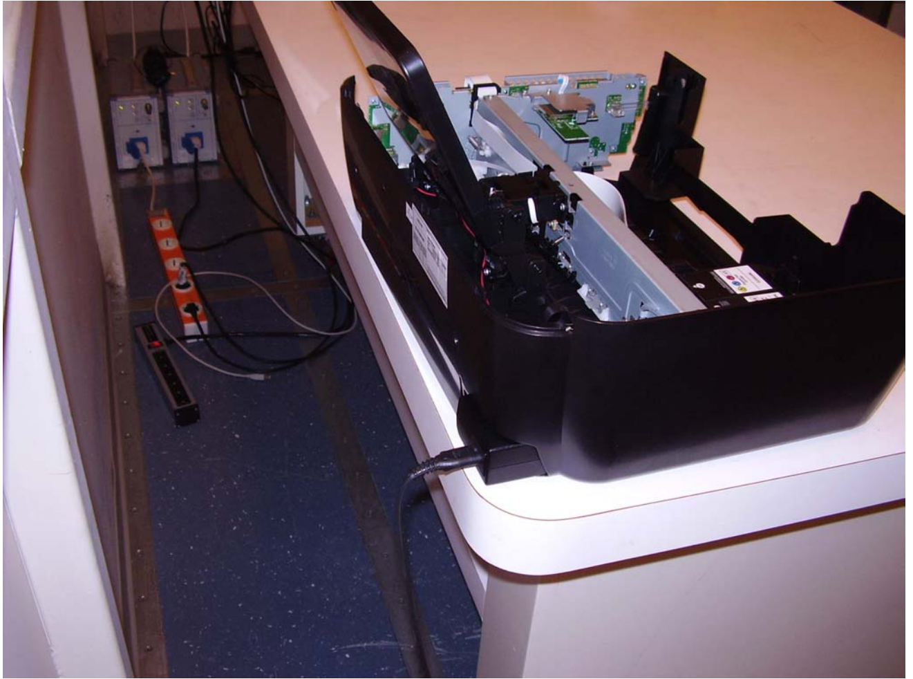
Test configuration for AC conducted emissions (side view).
