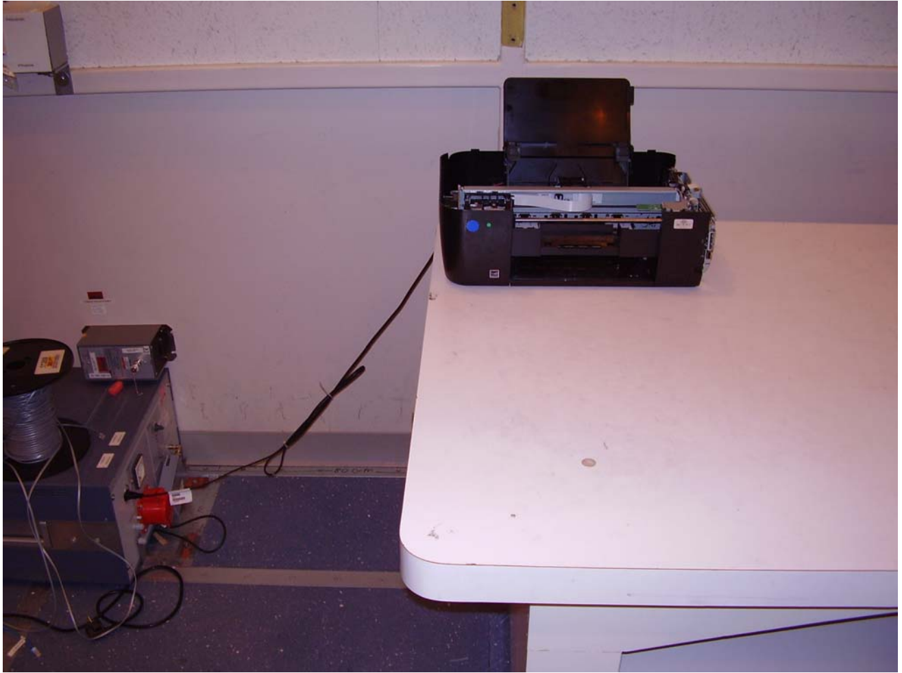
Test configuration for AC conducted emissions (front view).
