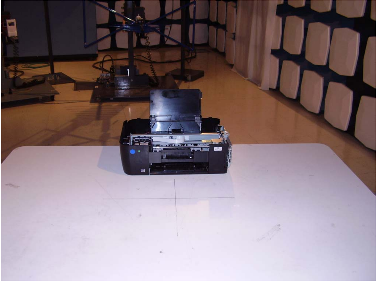
Test configuration for radiated emissions at frequencies > 30 MHz (front view).
