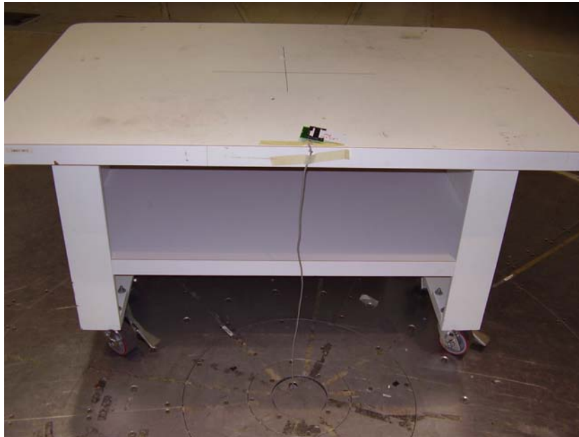
Figure 14. Test configuration for radiated emissions (back view).
