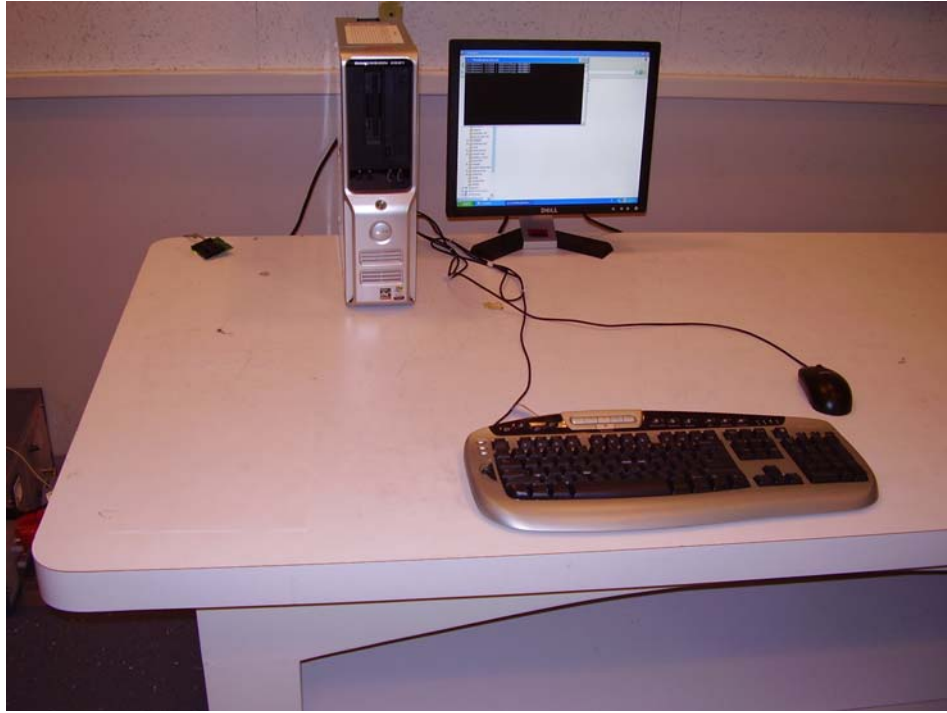
Test configuration for transmitter AC conducted emissions (front view).
