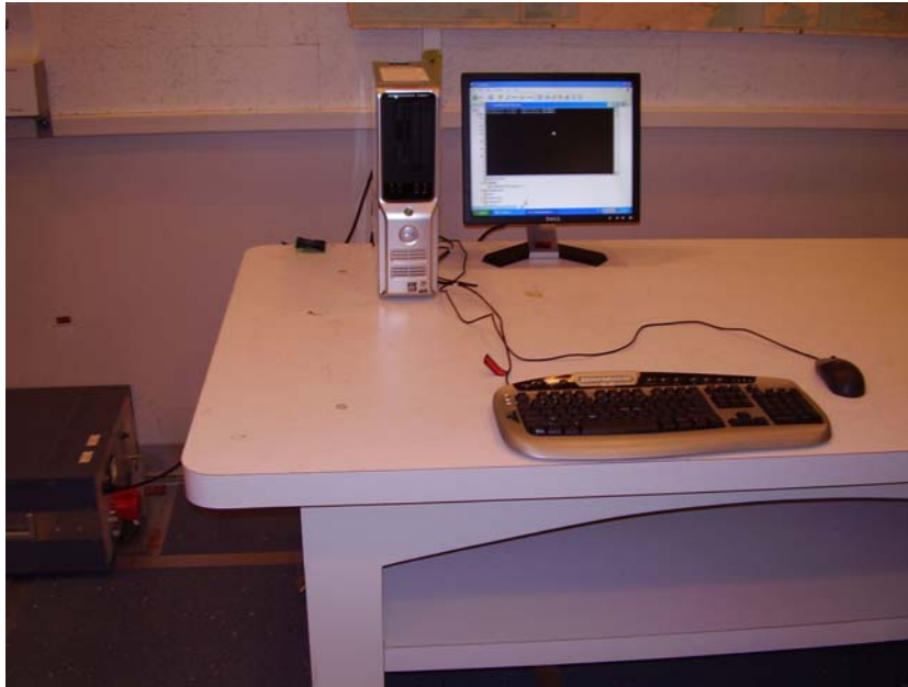
Figure 8. Test configuration for transmitter conducted emissions (front view).
