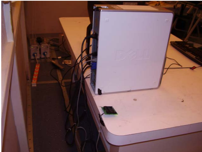
Figure 9. Test configuration for transmitter conducted emissions (side view).
