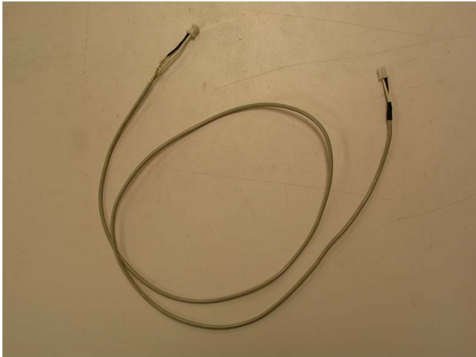
View of shielded cable between engine control board and antenna
