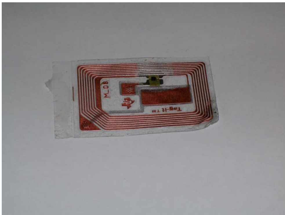
Transponder inlay from toner cartridge
