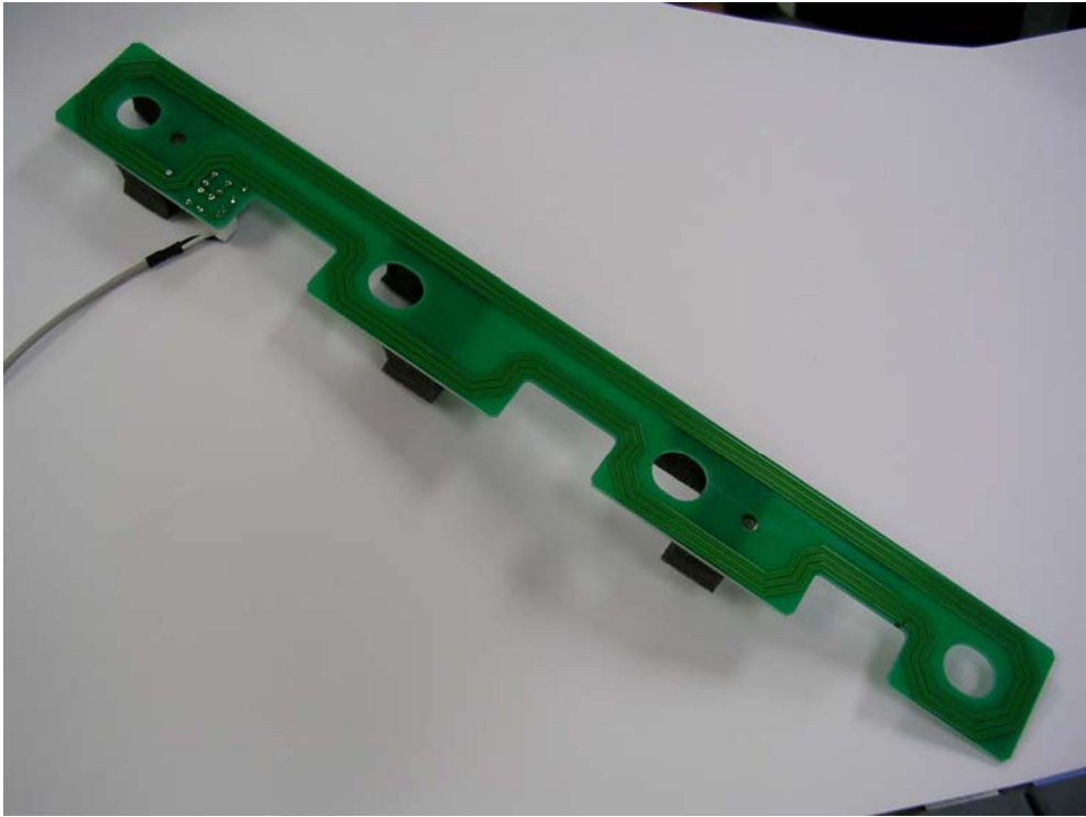
Detailed rear view of RFID antenna
